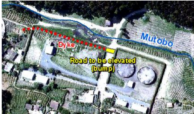
Figure 134 Location of the projected dyke
