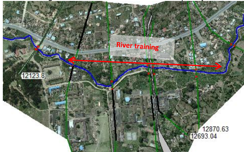
Figure 141 Proposed river training (HEC RAS cross sections in green)
