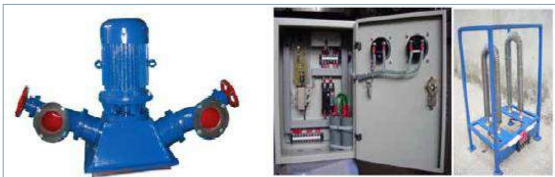
Figure 24: System components of the Power Pal T5 Hydropower package Vietnam (Meir and Fisher, 2011)
